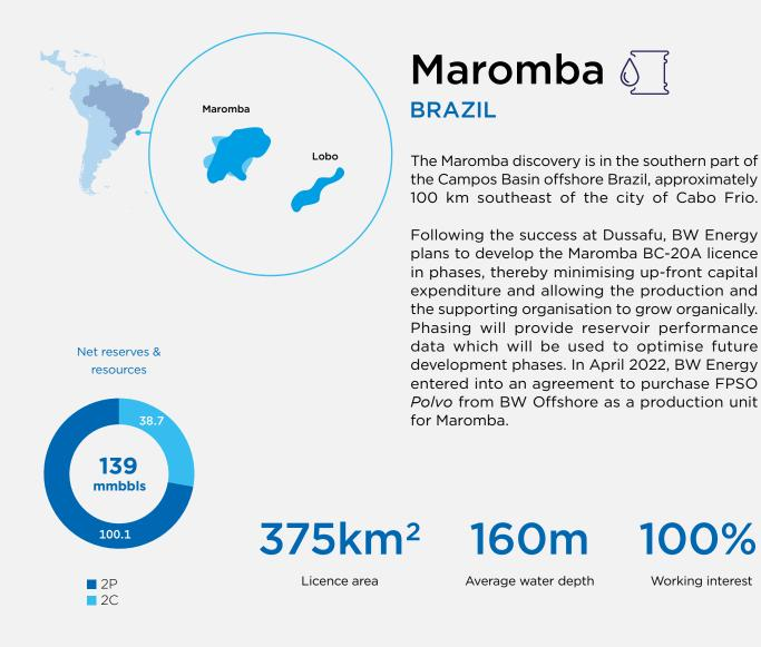
Phase 1 will target heavy crude oil at API gravity of 16° but with low relative viscosity and sulphur content in the Maastrichtian reservoir. It will consist of three horizontal subsea wells that will be tied back to FPSO *Polvo* with planned first oil in 2026. The wells will be completed with electric submersible pumps (ESPs) as the artificial lift mechanism.
